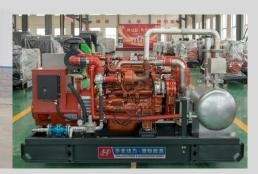
Its main equipment includes an engine, generator and heat recovery device. The working principle is that the biogas is supplied to the gas generator set by the storage tank through the desulfurizer, which drives the biogas internal combustion engine to generate electricity. The heat in the cooling water and exhaust gas discharged by the biogas generator unit can be recovered by the heat recovery device, and can be used as the heat source of the biogas generator.
